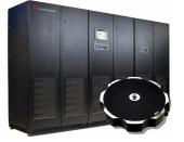
We market our flywheel-based UPS systems under the brand name CleanSource UPS rated at 300 kVA and 250 kVA for 480V and 400V applications, respectively. We currently offer CleanSource UPS products in power configurations ranging up to 1.5 MVA (million volt ampere) with the ability to parallel these products to provide even more protected power.
